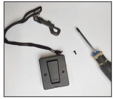
Use Philips head screwdriver to remove back panel and expose battery compartment.
