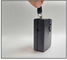
With the switch in the "down" position, test the alarm by pulling the pin. Alarm is very loud -- consider using hearing protection when testing.
