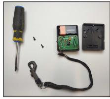
Install one 9v battery (not included) and replace back panel.
